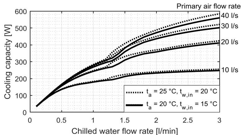
**Figure 15 Cooling capacity as a function of flow rates of chilled water and primary air, at two temperature levels.**
