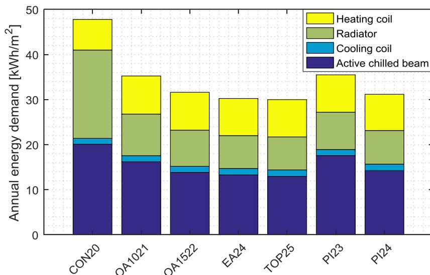
**Figure 20 Energy use with different strategies to control the supply chilled water temperature (CON20: Constant, OA: As a function of the outdoor air temperature, EA: As a function of the exhaust air temperature, TOP: As a function of the maximum operative temperature, PI: Non-self-regulating control).**
