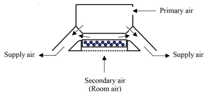
**Figure 2 Schematic diagram of an active chilled beam**
