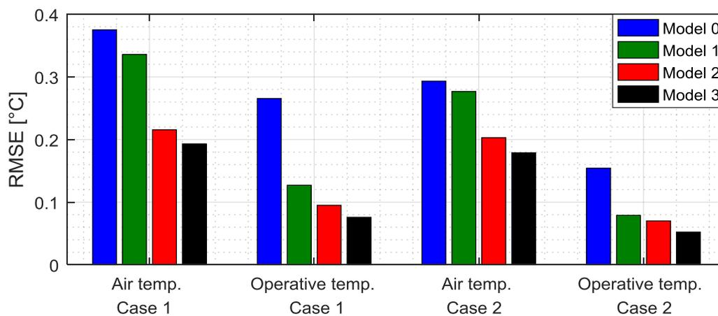
**Figure 16** Root mean square errors of simulated temperatures. Model 0 is the original default simulation, Model 1 takes thermal inertia of the sensors into account, Model 2 also takes induction into account and Model 3 also uses the supply air temperature as reference temperature.
