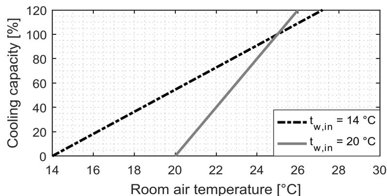
**Figure 5 Schematic correlation between room air temperature and cooling capacity of two active chilled beams with different chilled water temperature.**
