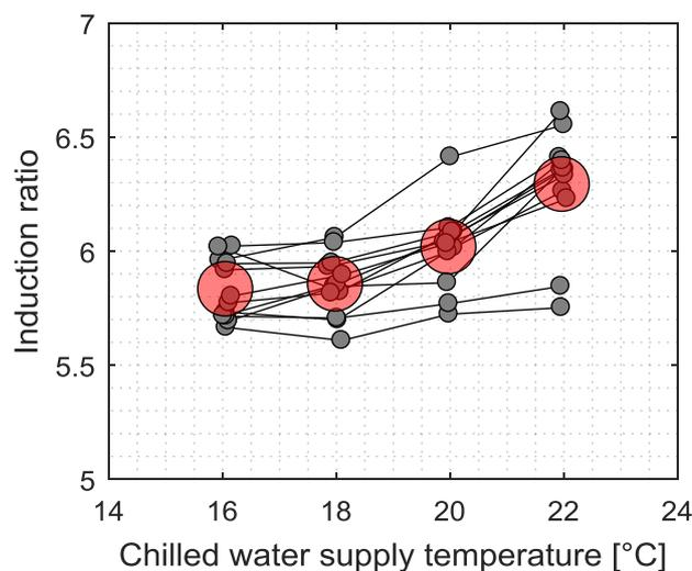
**Figure 14 Induction ratio as a function of chilled water supply temperature. Grey circles represent individual cases and red circles represent averages. Lines connect cases with equal internal heat gain, chilled water flow rate and primary air flow rate.**
