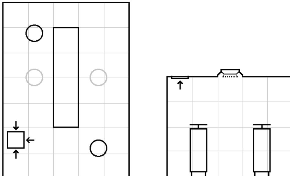
**Figure 12** Layout of the room and positions of active chilled beam, exhaust air terminal device and heat gain generators. Top view to the left and front view to the right. Grey lines indicate a distance of 0.6 m.
